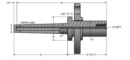
Maximum tapered length is 16" ("U" length for non-lagging wells) = "S" - 2" ("U" length for lagging wells) = "S" - 2" -"T" (To solve for "T"), "T" = "S" -"U" - 2" (When "U" and "S" are specified)
