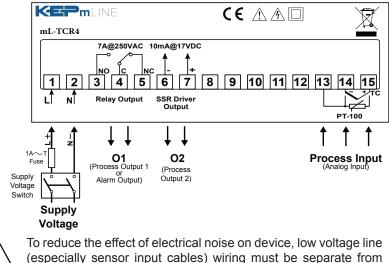
(especially sensor input cables) wiring must be separate from high current and voltage line. If possible, use shielded cable and shield must be connected to ground only on one side.
