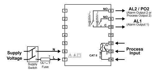
To reduce the effect of electrical noise on device, low voltage line (especially sensor input cable) wiring must be separetely from high current and voltage line. If possible, use shielded cable and shield must be connected to ground only one side.
