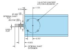
All dimensions are in inches with a tolerance of +0.005" or +0.01" unless otherwise specified
