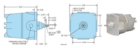
All dimensions are in inches with a tolerance of +0.005" or +0.01" unless otherwise specified
