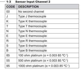
Process variable = the difference between Ch1 and Ch2
