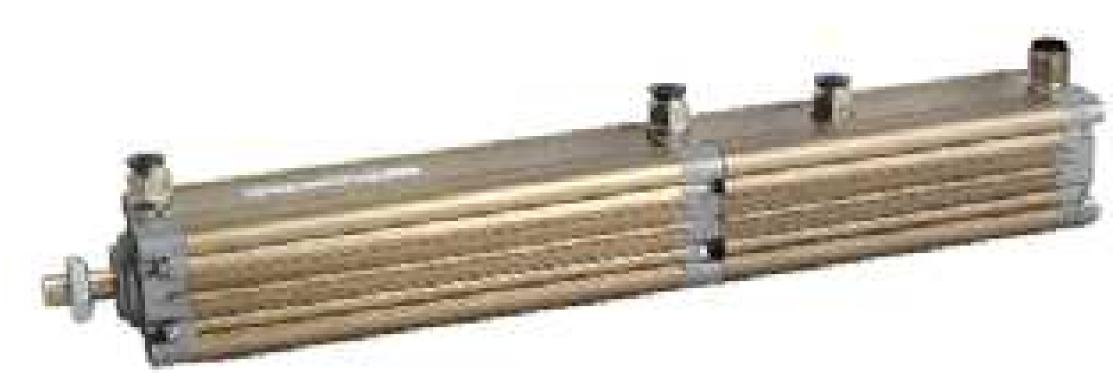
The system does not need to be connected to the moving part of the mechanism, as movement is generated by an internal piston with bidirectional pneumatic function. Such piston, operated by a 5-way valve, moves autonomously untill it meets the obstacle, thus measuring the stopping position.
