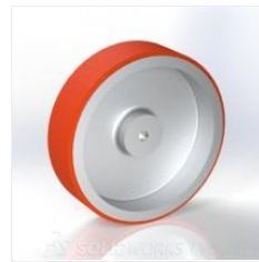
MW-1W-C 12" circumference measuring wheel, 1" wide, 1/4" bore
