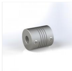
AE087-12-10 Flexible shaft coupling, 3/4"D x 1"L, 3/8" bore and 5/16" bore
