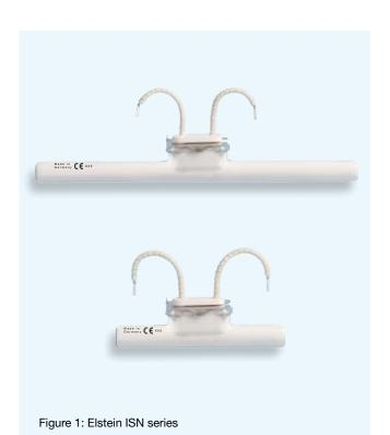
Elstein ISN rod radiators are ceramic infrared radiators, designed for surface ratings up to 72 kW/m<sup>2</sup> and operating temperatures of up to 750 °C.
