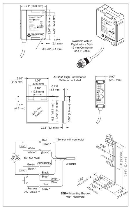
\*IMPORTANT: Sensor and Reflector must be mounted rigidly to insure proper operation.
