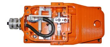
Cable routing: Route cable and solder wires to potentiometer in U shape, as shown (so as to assist in soldering leads to terminals). Secure with cable tie so wires cannot contact moving parts. Picture shows model G700-1K (note: this picture does not show the switch that is on the "-S" versions).
