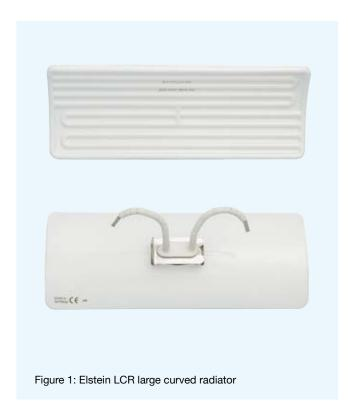
Elstein LCR large curved radiators are ceramic infrared panel radiators, which are designed for operating temperatures up to 750 °C. Surface ratings of up to 60 kW/m² can be installed.
