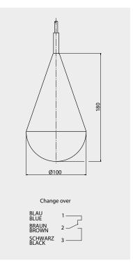
Type combination see type key Suspended Float Switches
