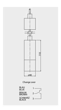
Type combination see type key Suspended Float Switches
