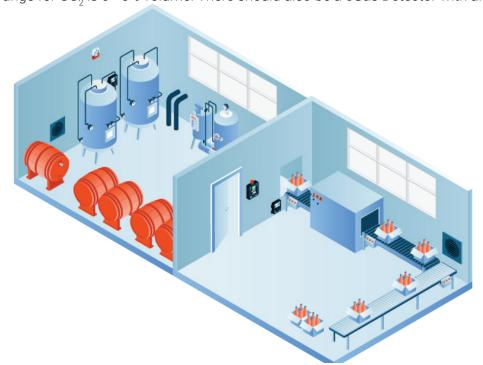
mounted on the wall near the  $\mathrm{CO}_2$  detector at the breathing zone height. It should be close to the fermentation tanks where oxygen is most likely to be depleted in the event of a build-up of  $\mathrm{CO}_2$ . The measurement range for  $\mathrm{O}_2$  is 0 - 25% volume. With the optional splash guard installed, both enclosures are water tight (IP54 rated) and will withstand water spray or wash down applications.
