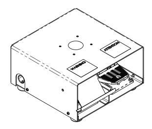
THE BGX500 INCLUDES ANY TWO GX-SERIES FOOT SWITCHES MOUNTED INSIDE THE STEEL ENCLOSURE WITH FOUR RUBBER BUMPER FEET. THERE IS A CONNECTION AREA INSIDE THE BACK OF THE COVER FOR WIRING AND A CABLE EXIT POINT OUT OF EITHER THE LEFT OR RIGHT SIDES.
