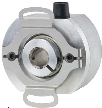
Encoders with 12-pole commutation and high temperature ratings (such as this EPC Model 260 slotted flex mount incremental encoder) are suitable for providing brushless servomotor feedback.
