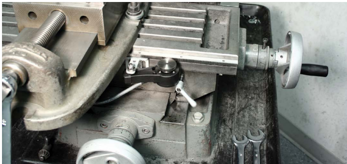
To enable precision feedback for reciprocating linear motion, the Model TR2 from Encoder Products Co. (EPC) eliminates backlash by integrating a pinion gear and rack.
