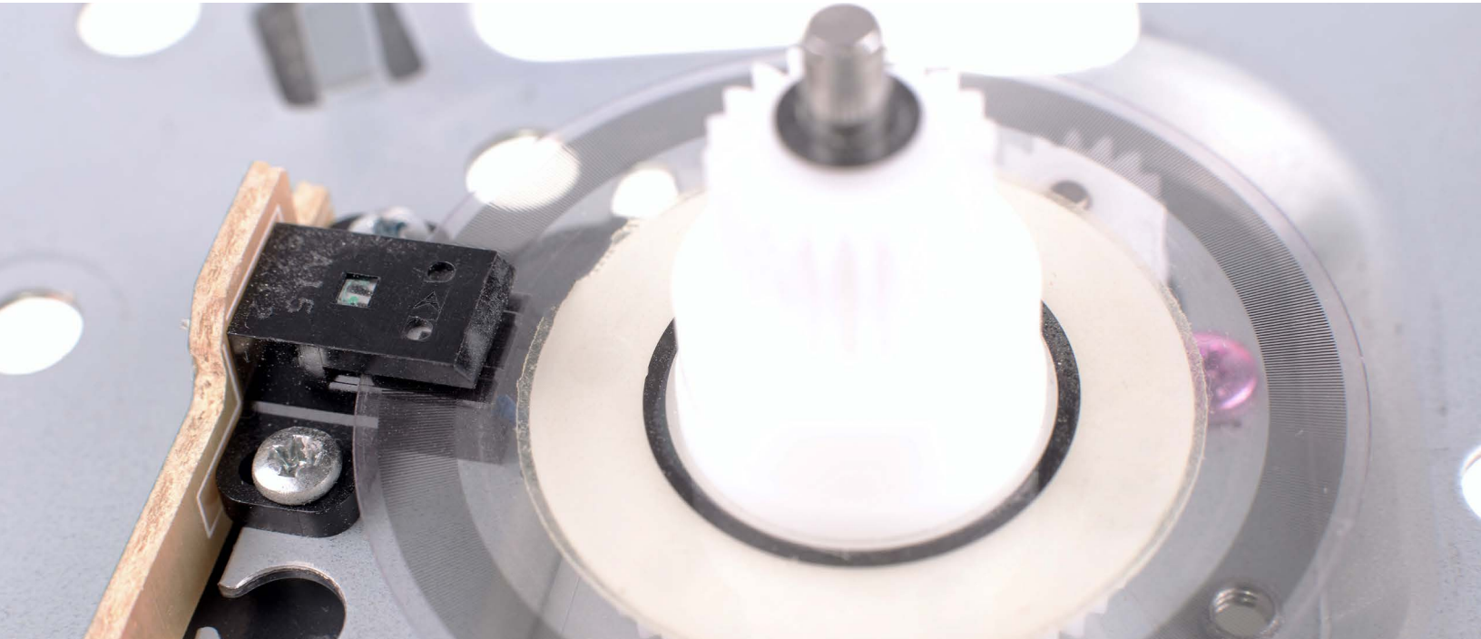
Shown here is the marked wheel of an optical encoder.
