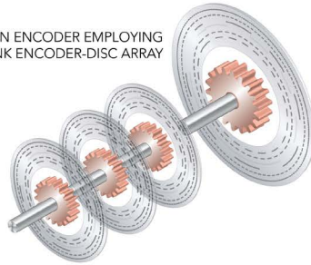
MULTITURN ENCODER EMPLOYING GEARING TO LINK PRIMARY FEEDBACK DISC TO TURN-MONITORING SECONDARY DISCS
