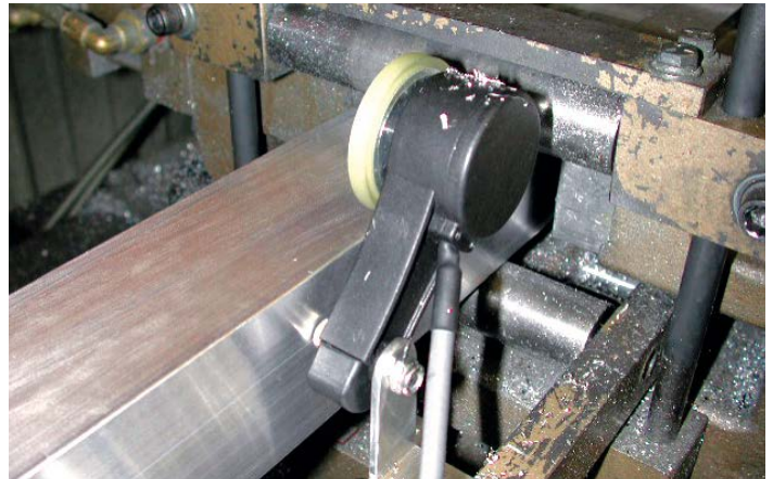
Wheeled encoders such as the Encoder Products Co. Model TR1 are well suited to metal-forming machines that execute extruding, profiling, and cut-to-length applications.
