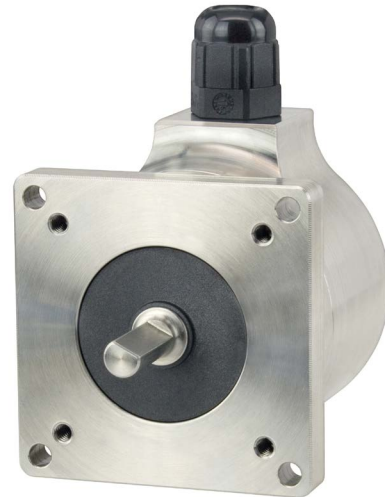
Where an encoder may be exposed to caustic chemicals or other harsh factory conditions, consider a stainless-steel unit with IP67 sealing. Shown here is one such Encoder Products Co. (EPC) Model 802S stainless-enclosed incremental-shaft encoder.
