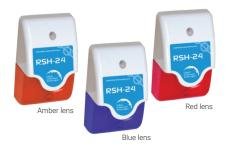
The Remote Strobe / Horn combines two alarm features, a visual and an audible into one compact, low profile device. It is powered by 24 VDC. The strobe and siren can be configured to activate together or each can activate separately from each other. It is recommended that this device be suitably mounted on a standard electrical box with conduit and protected from water ingress.
