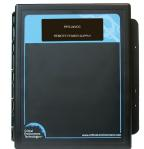
The RPS-24VDC is a remote power supply for large fixed system applications and/or very long wire runs. It converts 90 - 240 VAC power to 24 VDC power, providing a renewed amount of power to compensate for voltage drops. Projects requiring a large number of gas detectors or consist of very long wire runs require a remote power supply to boost the voltage to the last transmitter on the network run and to reinforce the voltage provided by the Controller to the first line of transmitters.
