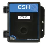
The ESH-A Remote Sensor offers flexible location monitoring of combustible or PID TVOC gases in non-hazardous, nonexplosion rated, commercial and light industrial applications. It communicates with a controller or transmitter using current loop into a 100 ohm load or a voltage signal of 0.40 to 2 volts.
