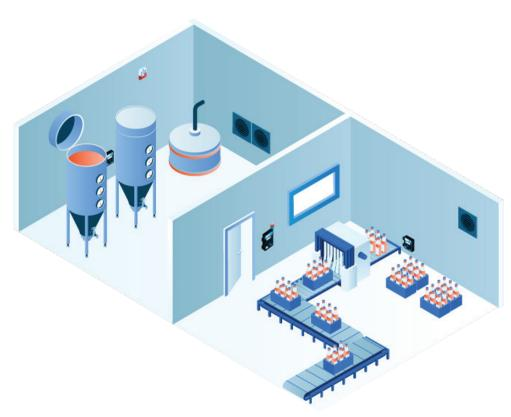
withstand water spray or wash down applications. During the bottling process, CO<sub>2</sub> is used to pre-fill each bottle before it is filled with beer. Another cGas Detector with a CO<sub>2</sub> infrared sensor should be mounted in the bottling area to monitor and protect workers on the bottling line.
