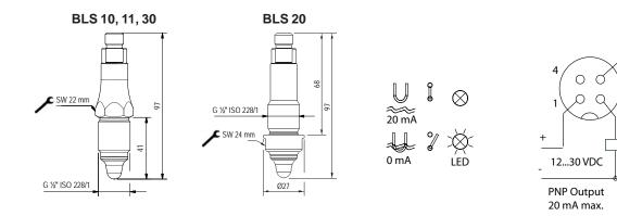
The tip of the sensor is made of PEEK plastic. The sensor works on the principle of frequency-sweep technology. The sensor output can be switched from digital to pulse width modulation (PWM). The sensor recognizes different media and can therefore be used for media separation. The analysis of the PWM signal must be done in the connected control unit (PLC).
