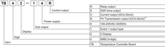
X1: PV transmission output type does not have Event 1 output.
