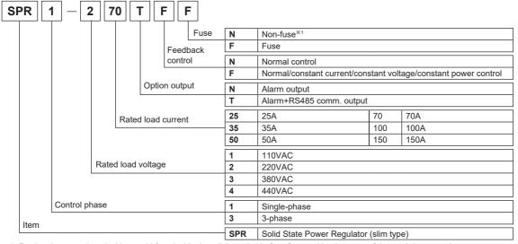
※1: Product is not equipped with a rapid fuse inside. Install the suitable fuse for rated load current of the model separately.
