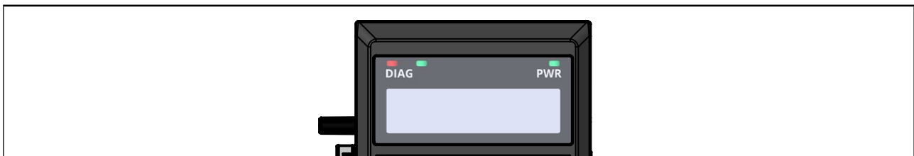
Figure 32: LED display of a valve unit
