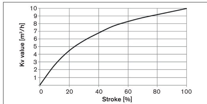
Fig. 20: Flow characteristic for orifice 20 ( \varnothing 50 )
